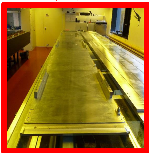
Figure 48 Alignment of the Panel side bracket
