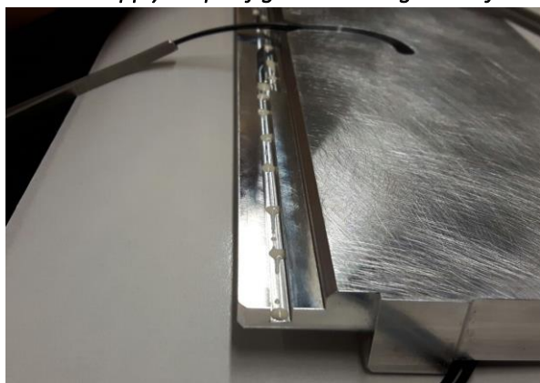
Figure 19 Glue in groove for light bar
