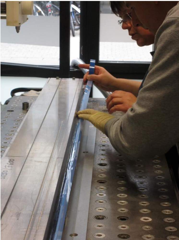
Figure 28 Tape on cut sides of the mats
