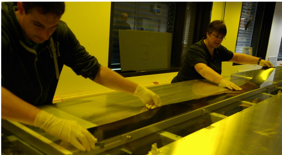
Figure 37 Placing mats to the gluing jig
