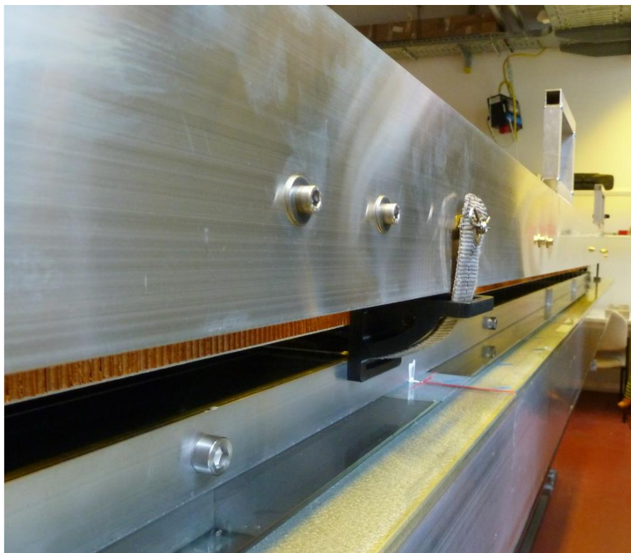
Figure 55 “Security belt” attached to the “Lifting and Turning device”.
