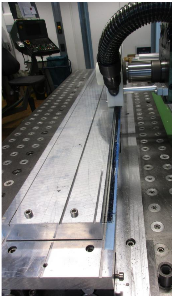
Figure 29 Cutting one side of the mat
