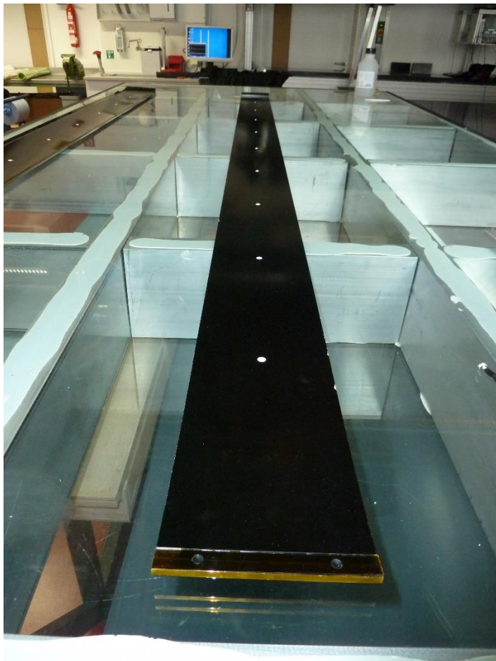
Figure 3 SciFi mat with mat pins up
