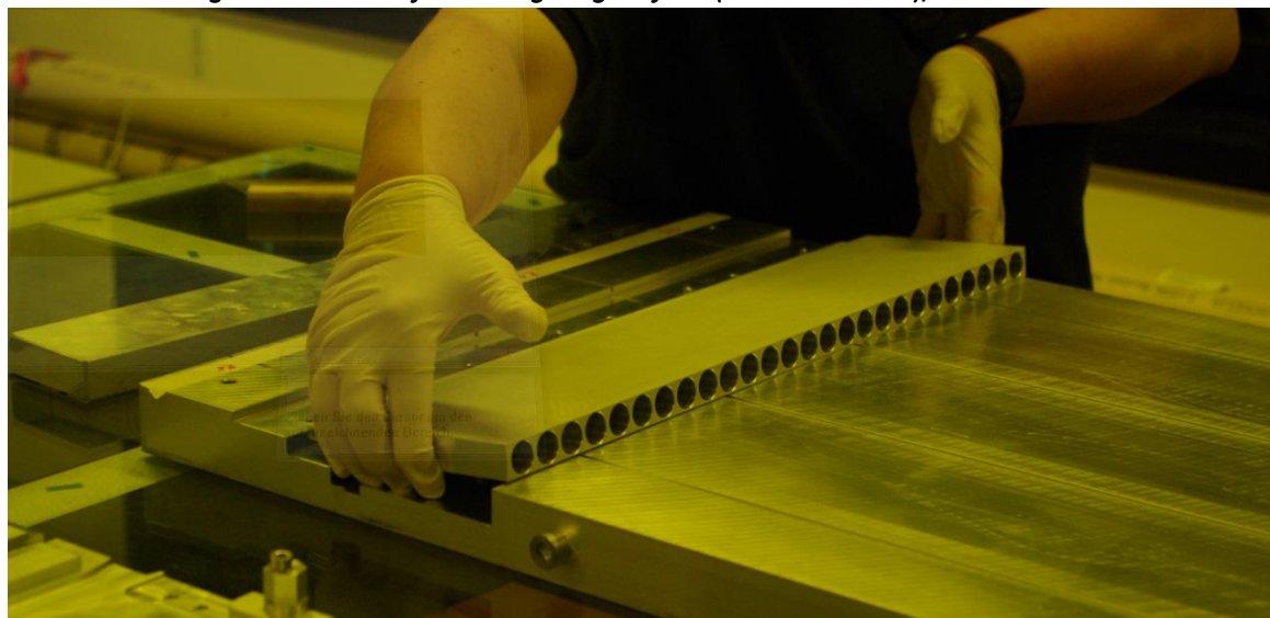
Figure 35 Endplug in gluing jig
