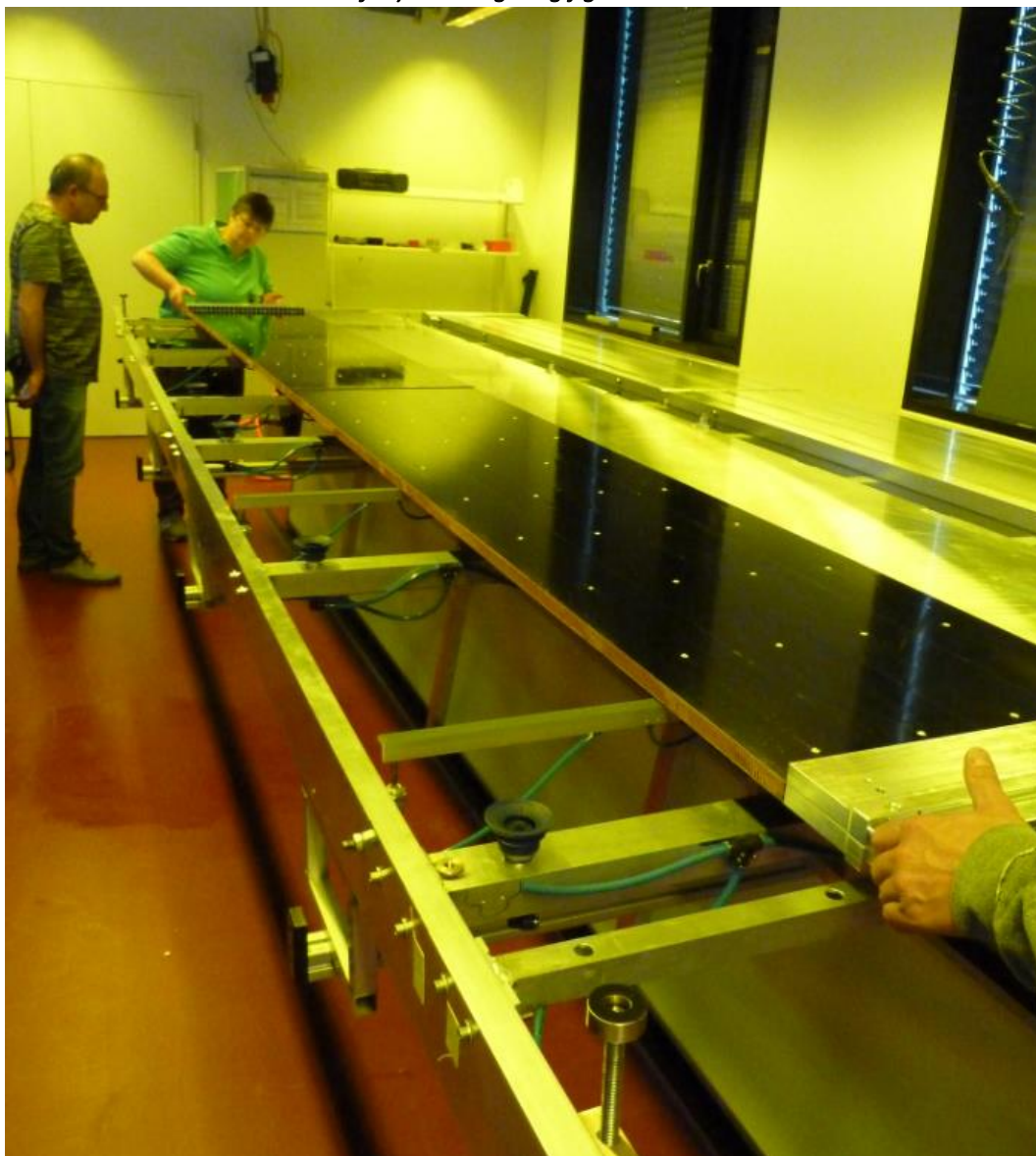
Figure 59 Half module been pushed on the gluing jig
