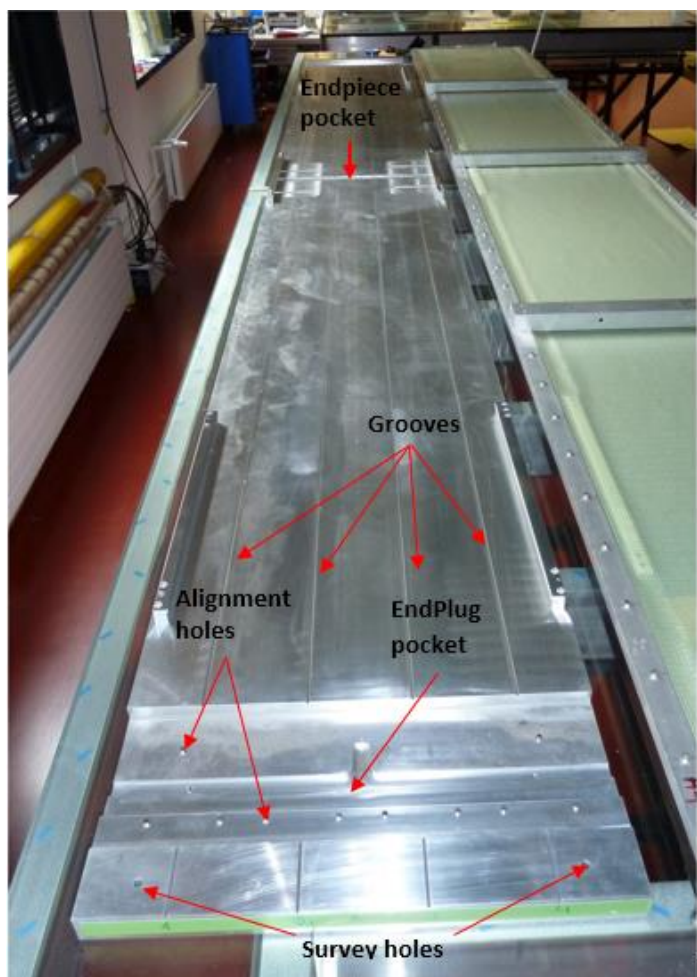
Figure 7 Overview gluing jig
