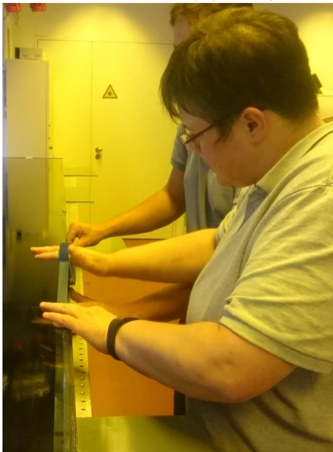
Figure 65 PET-tape to avoid the glue spreading out
