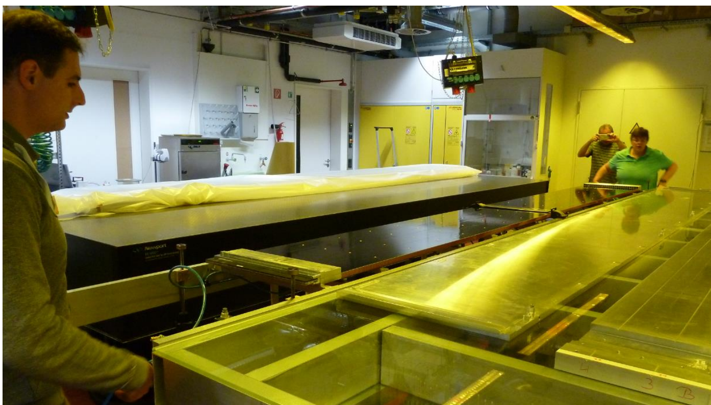
Figure 58 "Lifting and Turning device" with half module turned and placed next to the gluing table
